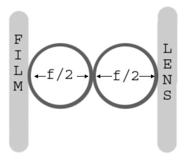
Diameter is 1/2 the distance between film and back end of lens
