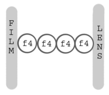
Diameter is 1/4 the distance between film and back end of lens
