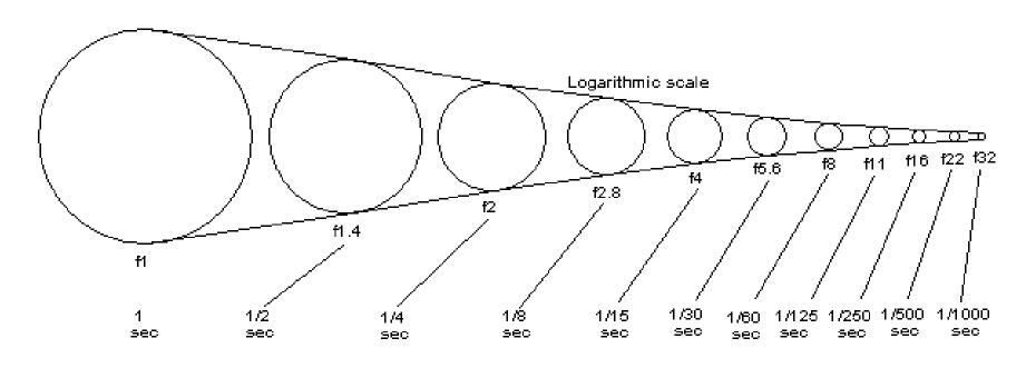
The above equates aperture and time as equals with regard to effect on exposure - i.e., be aware that each halving of time equates to a halving of aperture cross-sectional area, and thus, each step of halving (or doubling) has the same effect on the light transmitted to film. For example - a reduction of f2 to f2.8 causes a halving of light transmitted, as would a reduction in exposure time from, say, 1/4 sec to 1/8 sec.
