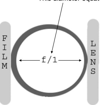
Diameter is 1/1 the distance between film and back end of lens
